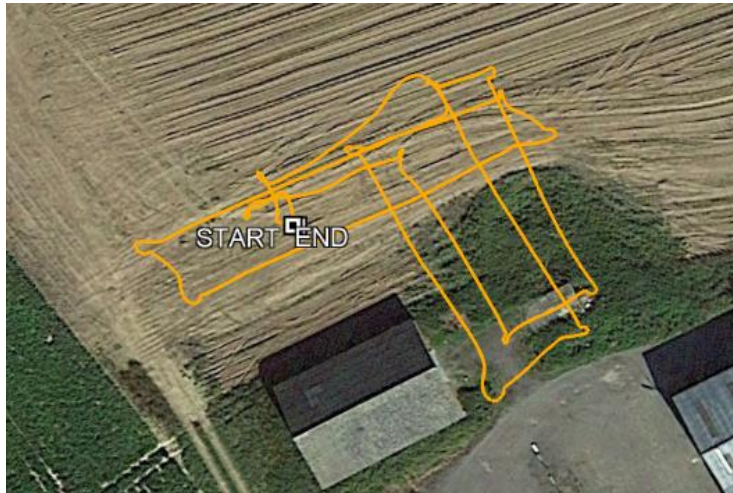
Figure 9: Trajectory of the UAV test flight, showing multiple passings of the barn (bottom) and concrete slab (right of the barn).
