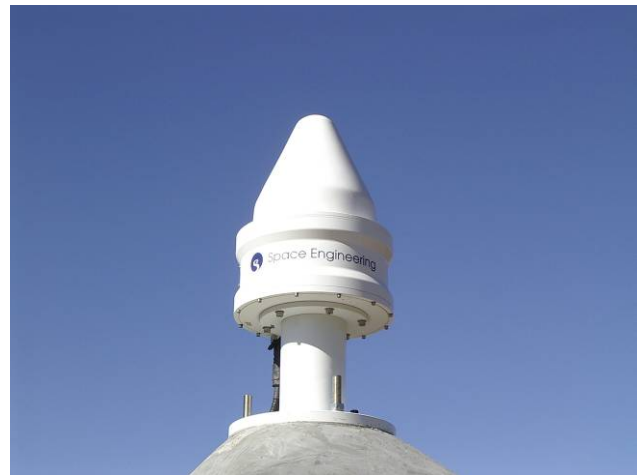
Figure 4. The wide-band Space Engineering antenna, which was used in this work, allows reception of GPS L1, L2 signals as well as Galileo L1, E5, E6.
